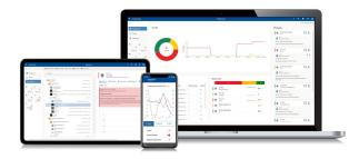
The Plantweb Optics Asset View provides a KPI dashboard view of monitored assets and alerts you to developing issues on the assets you define as critical to your production. The interface is similar across desktop/tablet/smart phone views for ease of use, while the mobile app provides a multi-site view for easy review of alerts across the enterprise. Drill down on individual assets to understand why assets have degrading health scores.
