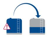
Overfill Prevention - Maintain an incidentfree operation by accurately tracking product on board and the exact amount that can be loaded based on compartment capacity (physical overfill protection devices are still required).
