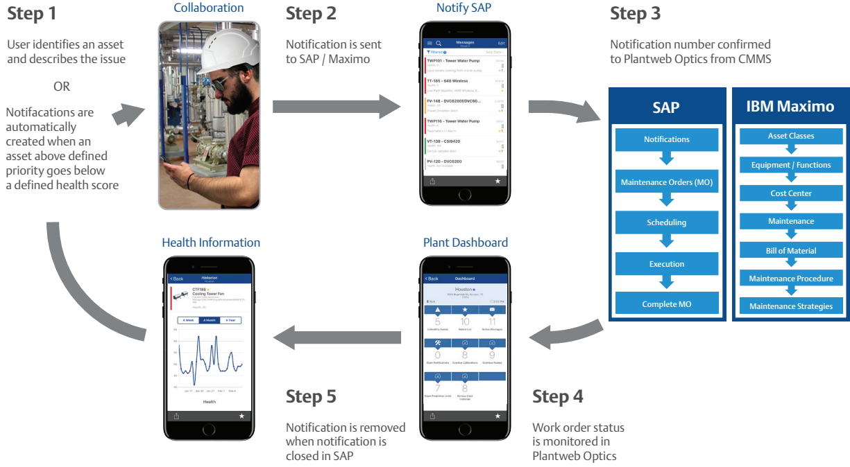
The workflow process with the Plantweb Optics CMMS interface.
