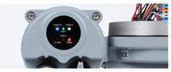
Including a local control station with an HQ actuator provides a quick and easy way to check actuator status and control operation. LCUs, depending on model size/type, offer a variety of controls and displays. LCUs can be as simple as two selector knobs for open/close control, or with indication LEDs, or with a Liquid Crystal Display showing digital valve position.
