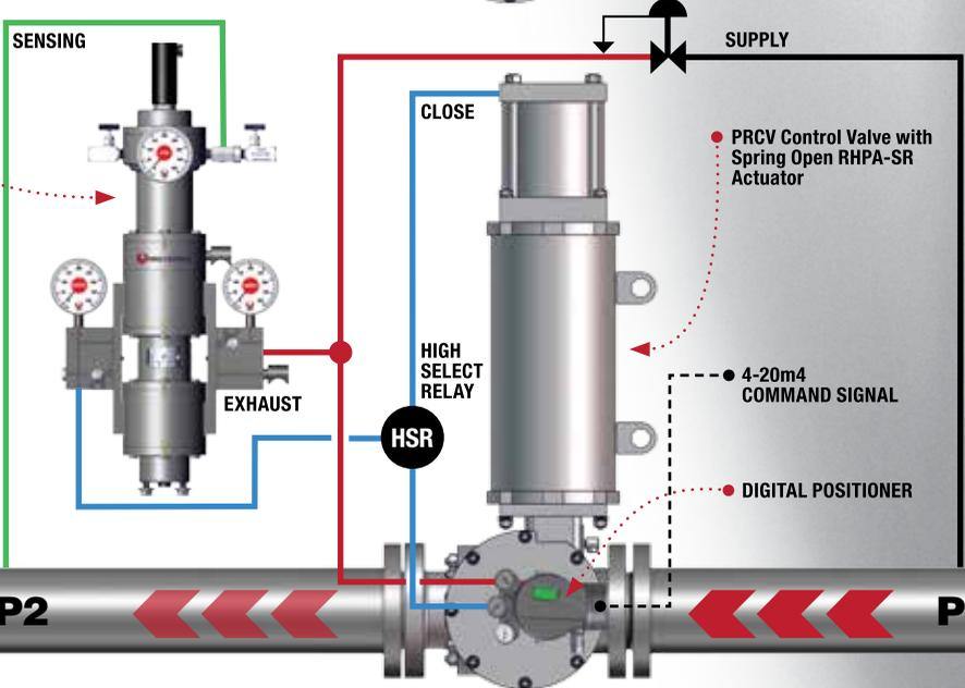
PRCV Control Valve with Spring Open RHPA-SR Actuator
