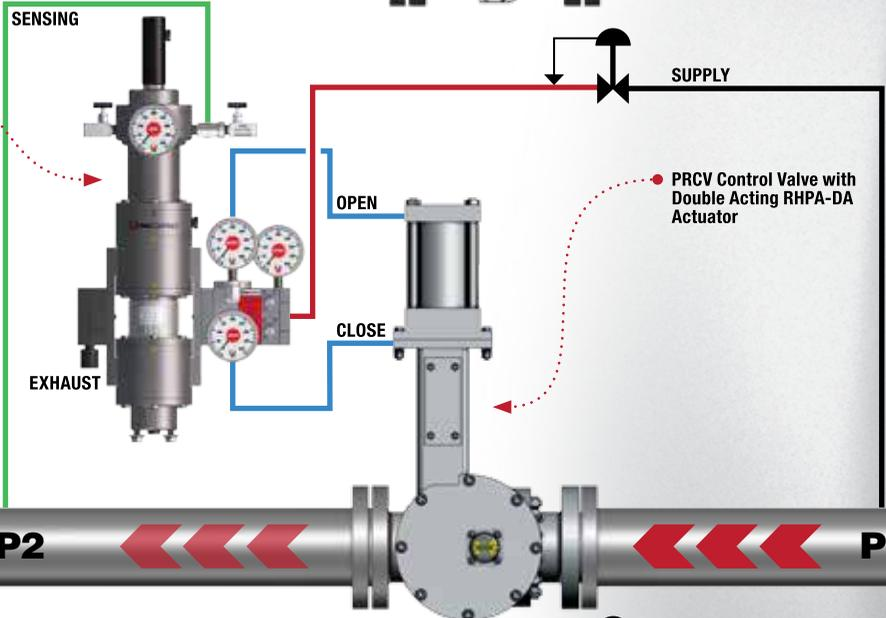
PRCV Control Valve with Double Acting RHPA-DA Actuator
